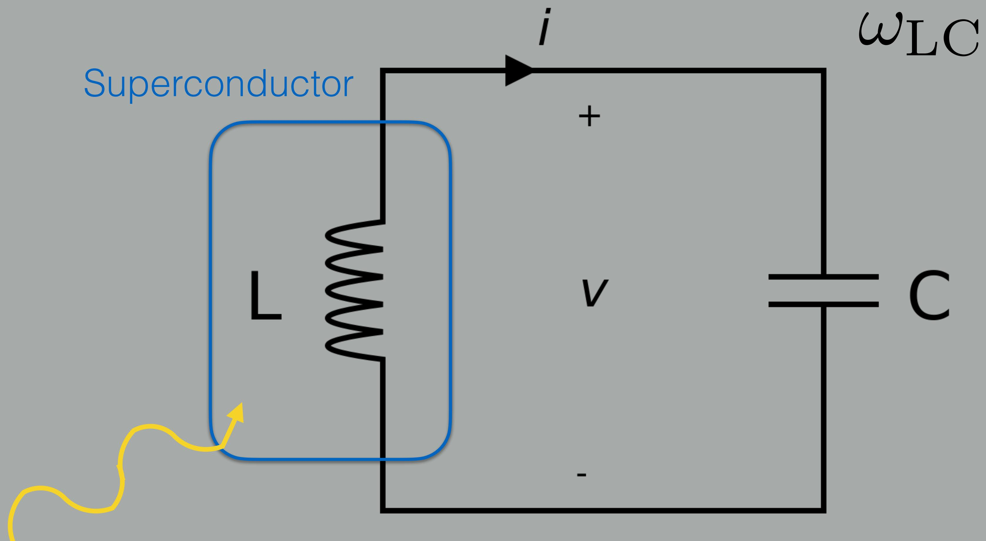
Photon absorbed by superconductor reduces kinetic inductance, altering the resonant frequency of the LC circuit
