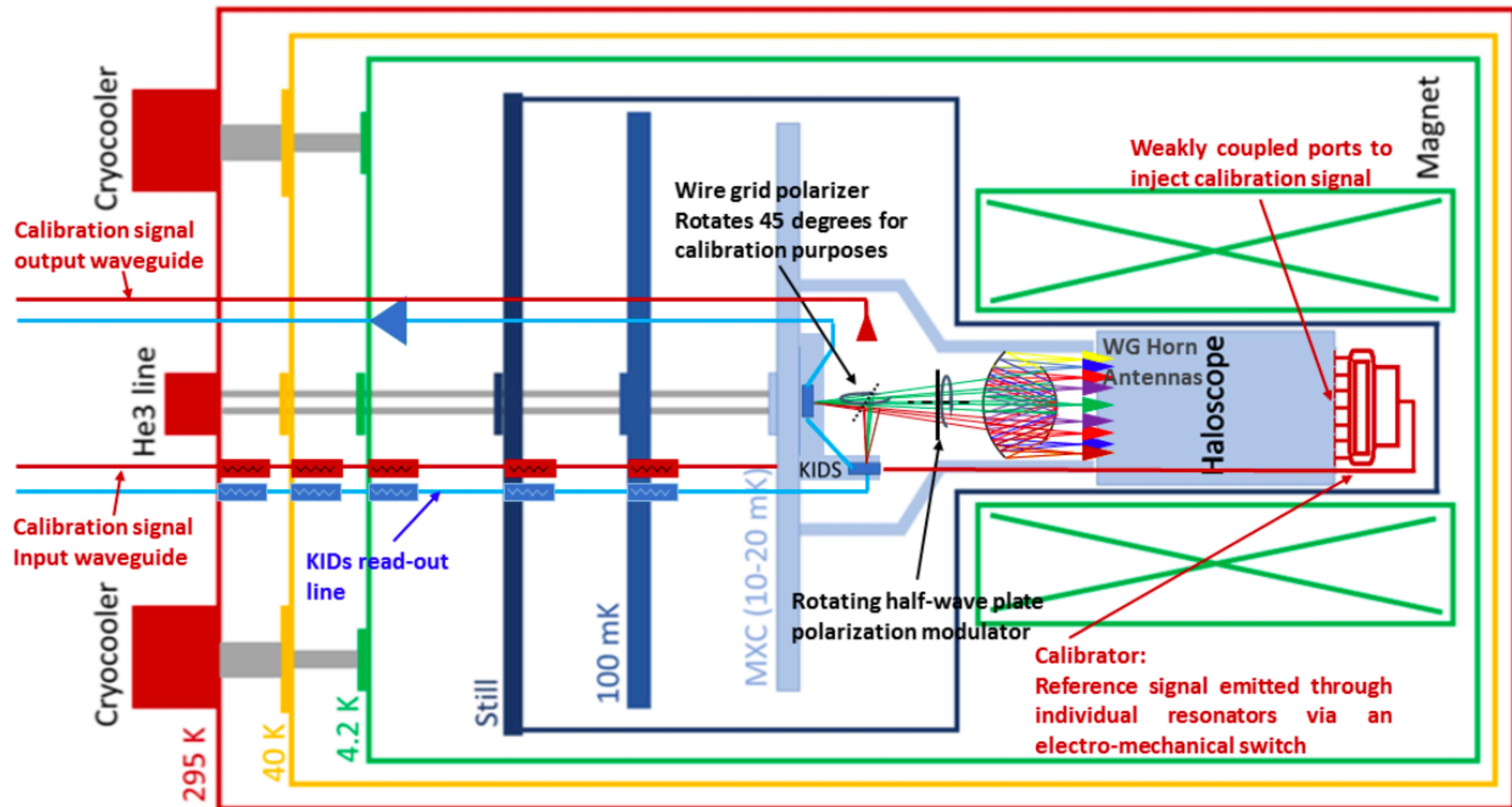
Immerse haloscope array in high static magnetic field of  $B = 8\text{-}10 \text{ T}$
